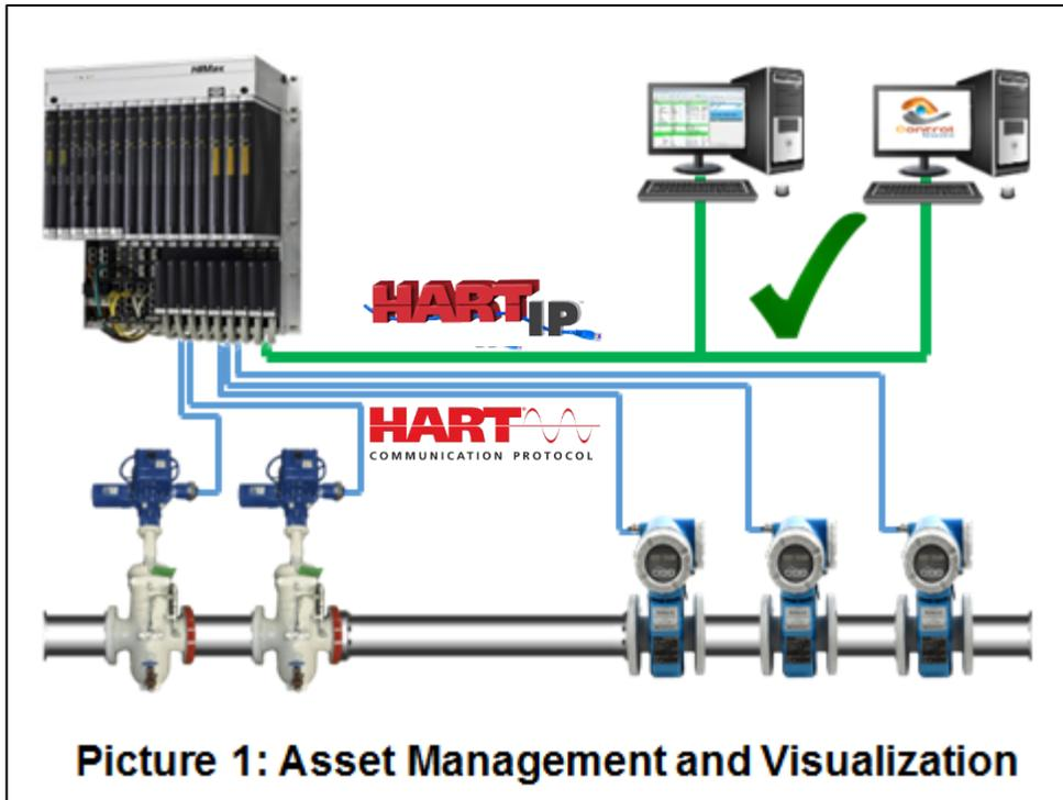
When HART devices are used in safety instrumented functions (SIFs), the HART information is often totally overlooked, and the primary usage of the HART capability becomes to allow for calibration via a handheld calibrator. It should be noted even this innocent use of the HART protocol creates a risk. Any technician can re-configure the HART device which could render the SIF totally ineffective.
